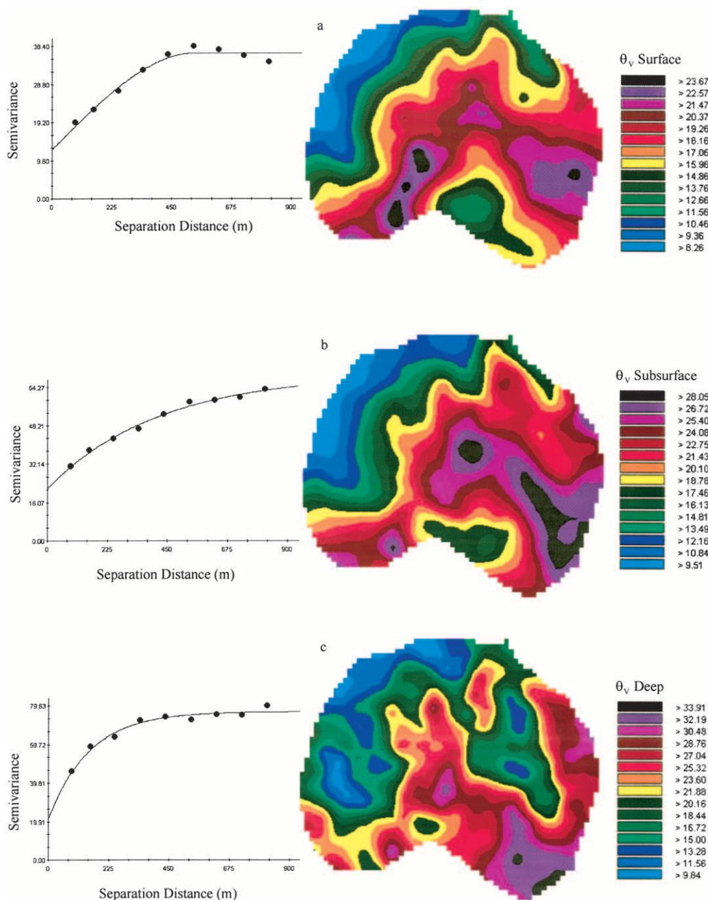
Fig. 7. Semivariograms and kriged maps of volumetric water content ( $\theta_v$ ),  $\text{cm}^3 \text{cm}^{-3}$ , expressed in percentage at wilting point (equivalent to  $-1500 \text{ kPa}$  pressure head) for the (a) surface, (b) subsurface, and (c) deep horizons.
