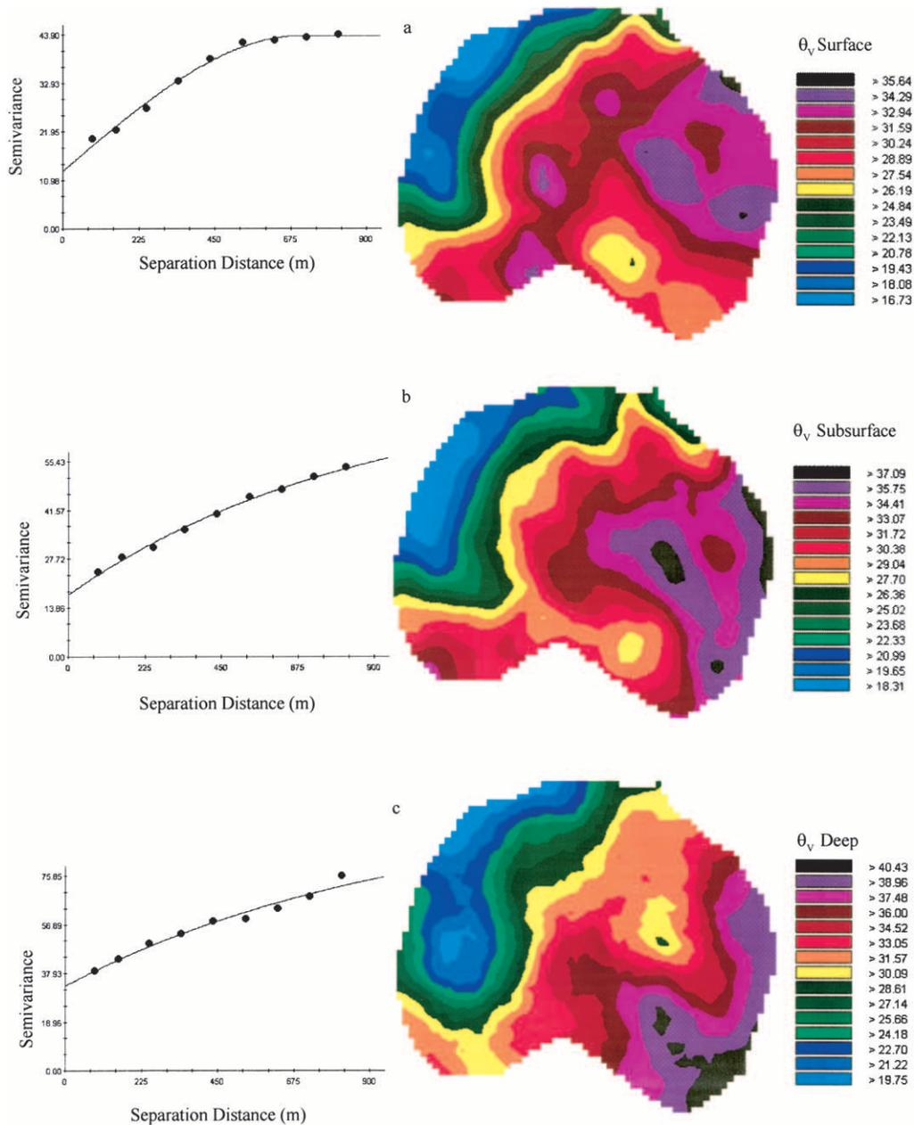
Fig. 6. Semivariograms and kriged maps of volumetric water content ( $\theta_v$ ),  $\text{cm}^3 \text{cm}^{-3}$ , expressed in percentage at field capacity (equivalent to  $-33 \text{ kPa}$  pressure head) for the (a) surface, (b) subsurface, and (c) deep horizons.
