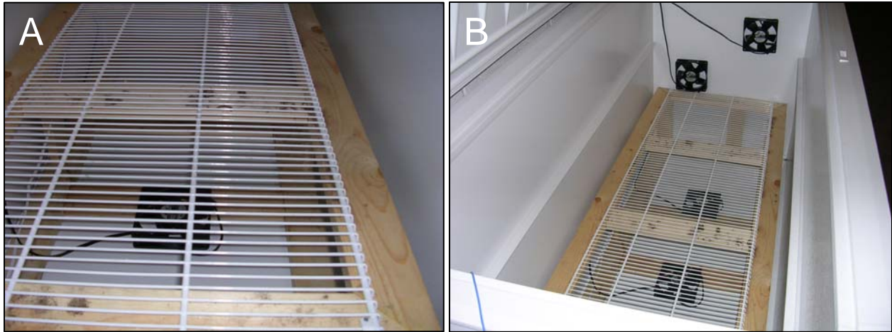
Figure 1. Vinyl shelving was used to construct flooring for the base of the freezer and computer case fans were attached with Velcro and used to circulate air within the chamber.
