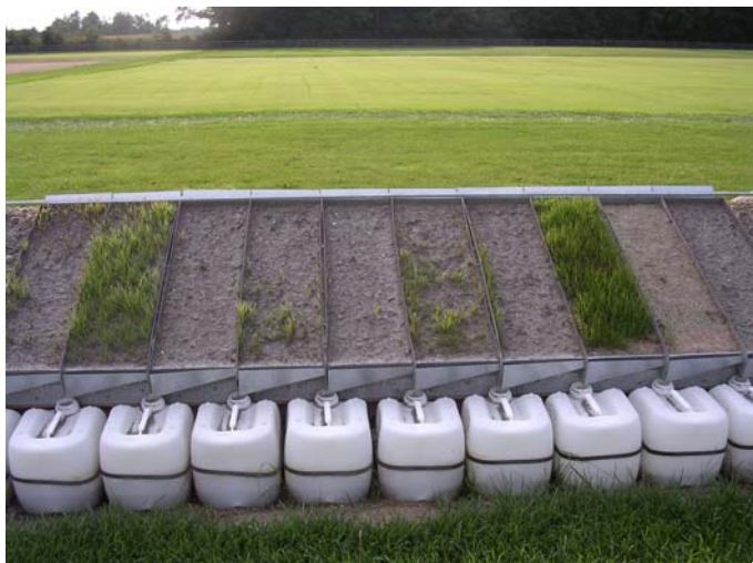
Figure 2. Promising grass species identified in 2005 were planted on runoff slopes containing dredged and sandy soil in the summer of 2006.
