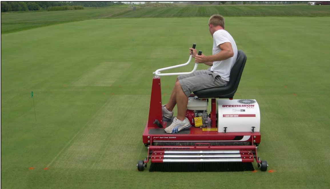
Figure 2. Roller/brush treatments were conducted as recommended by the manufacturers of the greensIRON 3000TM. Dragging the brush for the initial pass, then leading with the brush for the final pass.
