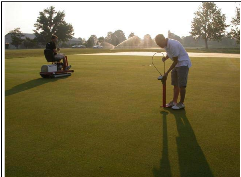
Figure 1. Overview of preparation procedures, repeated rolling and surface hardness measurements used to create the “firm” study area, 12 June, 2007.
