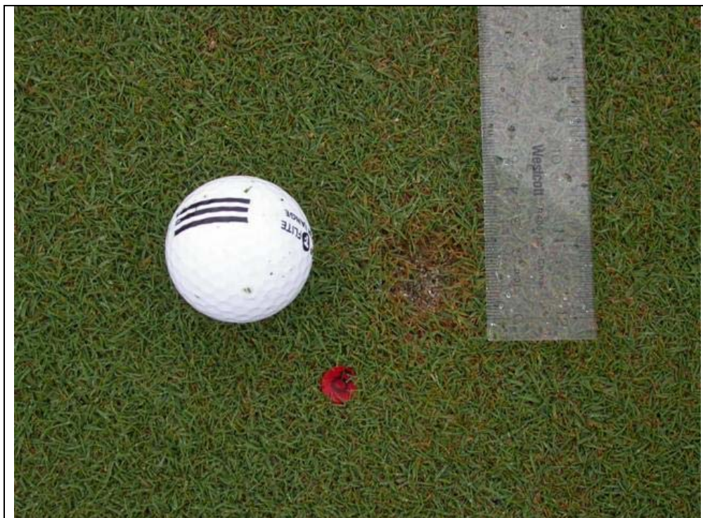
Figure 3. Overview of the method used to determine ballmark diameter and ultimately ballmark scar area. The numbered red tee indicates the treatment and replication number.
