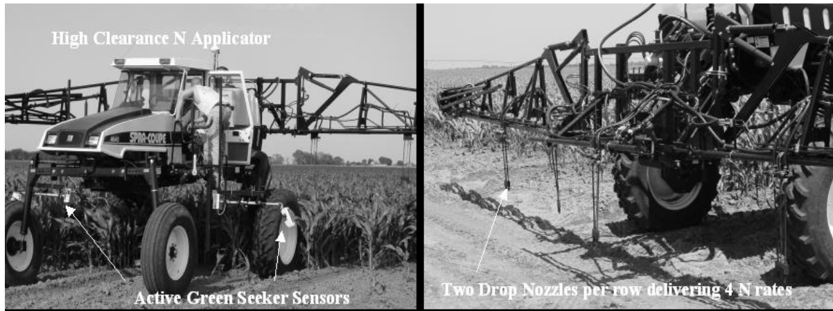
Figure 3. The high clearance N applicator (left) illustrating key components, including the active Green Seeker crop canopy sensor mounted on front. Both the red and green versions of the active sensor manufactured by Ntech Industries, Inc. ( http://www.ntechindustries.com/ ) were tested and evaluated. The liquid N fertilizer delivery system (right), consists of two drop nozzles/valves placed at alternating rows of corn. Depending on the configuration of valves turned on/off, the system can deliver multiples of four (i.e., (0, 45, 90, 135 kg N/ha) rates of liquid N fertilizer on-the-go as directed by the controller system interfaced to the active sensor or with a prescription map.
