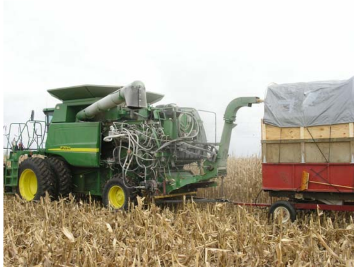
Figure 4. A prototype one-pass grain and stover combine developed by Dr. Birrell at Iowa State University, Ames, IA.
