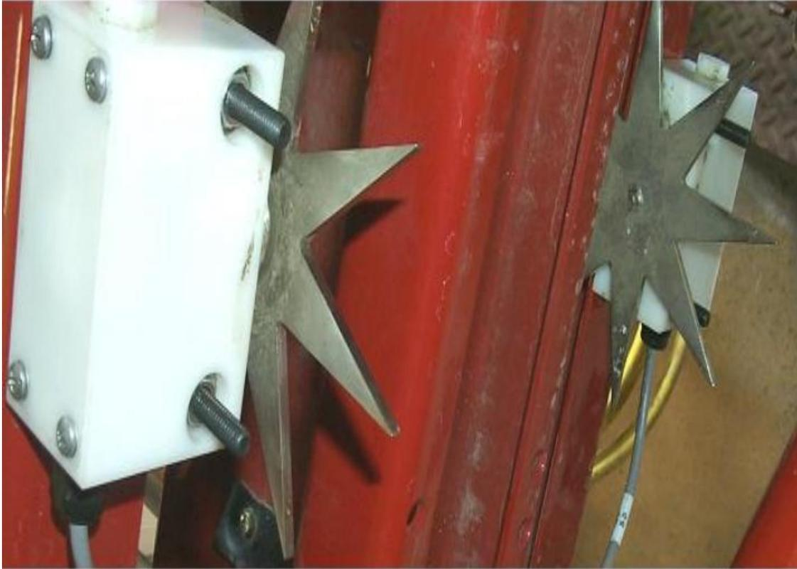
The 2 star wheel sensor is also used on conventional square bales. Because these wheels take so many readings and because they sense across a large distance, they provide accuracy within several points of a reading that would be taken using a coring tools and an oven.
