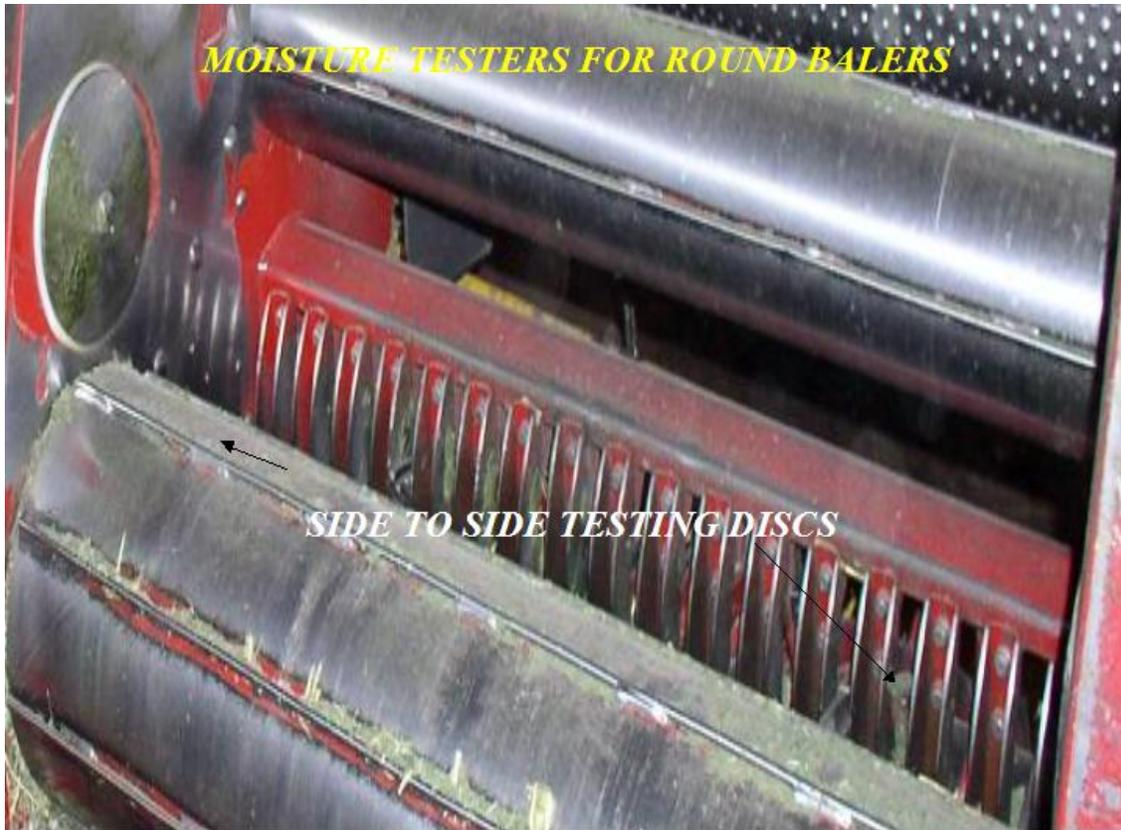
These accurate moisture-testing devices are the heart of Harvest Tec's automatic application systems. The systems are set to automatically turn the application on at 16% for large square bales, and 18% for conventional and large round bales. Automatic systems are not running all of the time. When they are on, they are adjusting application rate to moisture content of the hay, making an
